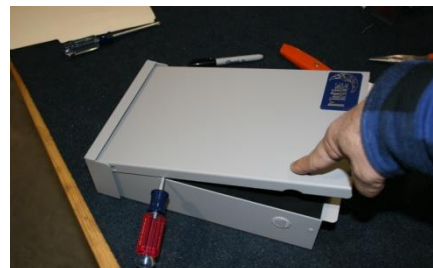
Remove top cover prior to removing the deadfront on Type 3R units.
