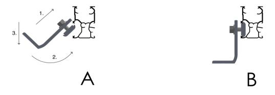
Figure 2: Inserting K-Nut into Side Channel
