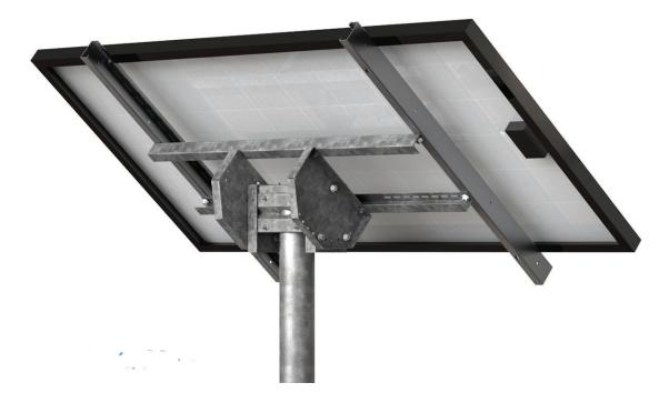
The STP-SCR/45R is designed and engineered for a single 60 or 72 cell module that is less than 45" wide. Mounts are manufactured using pre-galvanized steel and heavy-duty corrosion resistant 5000 series aluminum.
