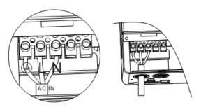
③ Properly connect the AC output wire according to the wire sequence and terminal position shown in the figure below. Please connect the ground wire first, and then the live wire and the neutral wire. The ground wire is connected to the grounding screw hole on the cabinet through the O-type terminal.
